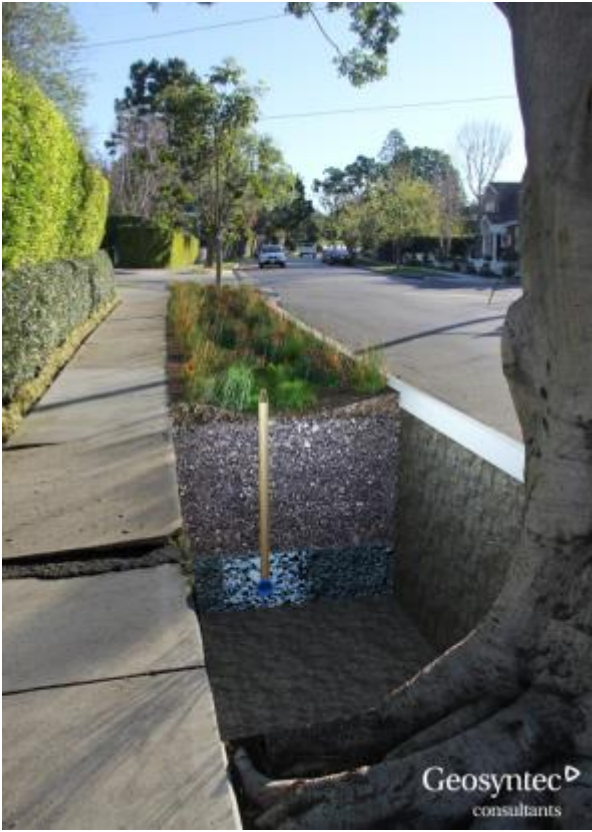
Figure 4-22 Section View of Bioretention with Underdrain
