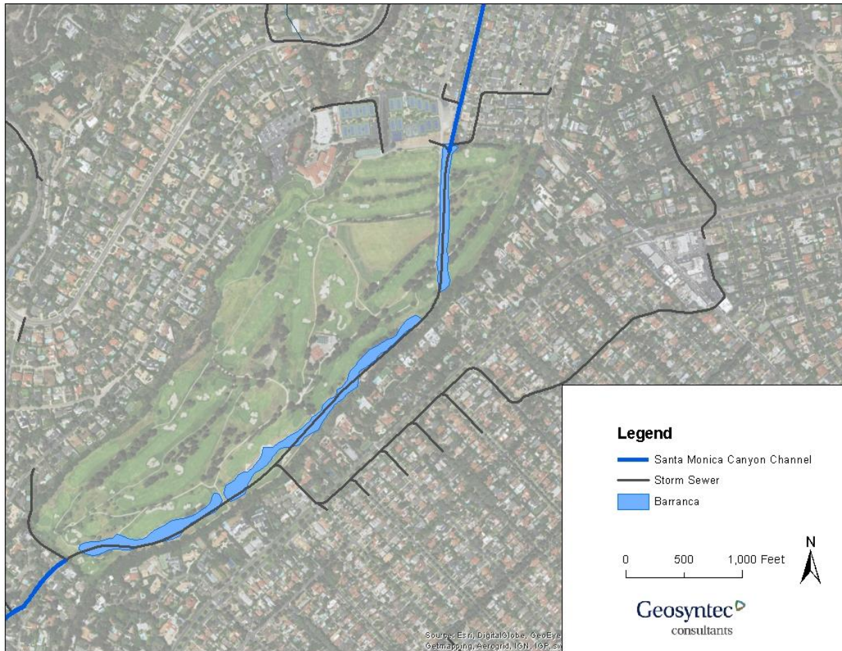
Figure 4. Stormwater infrastructure adjacent to the Riviera Country Club.
