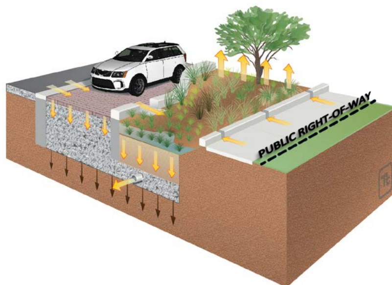
Figure 4-24 Typical Distributed Permeable Pavement Schematic with Underdrain
